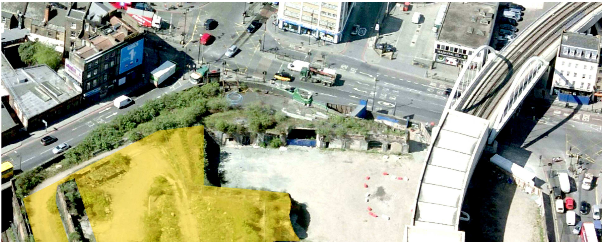
EXISTING BIRD'S EYE VIEW FROM SOUTH EAST - Southern and Western Arches (highlighted yellow) are to be removed leaving the Oriel Gateway as a stand alone building.
